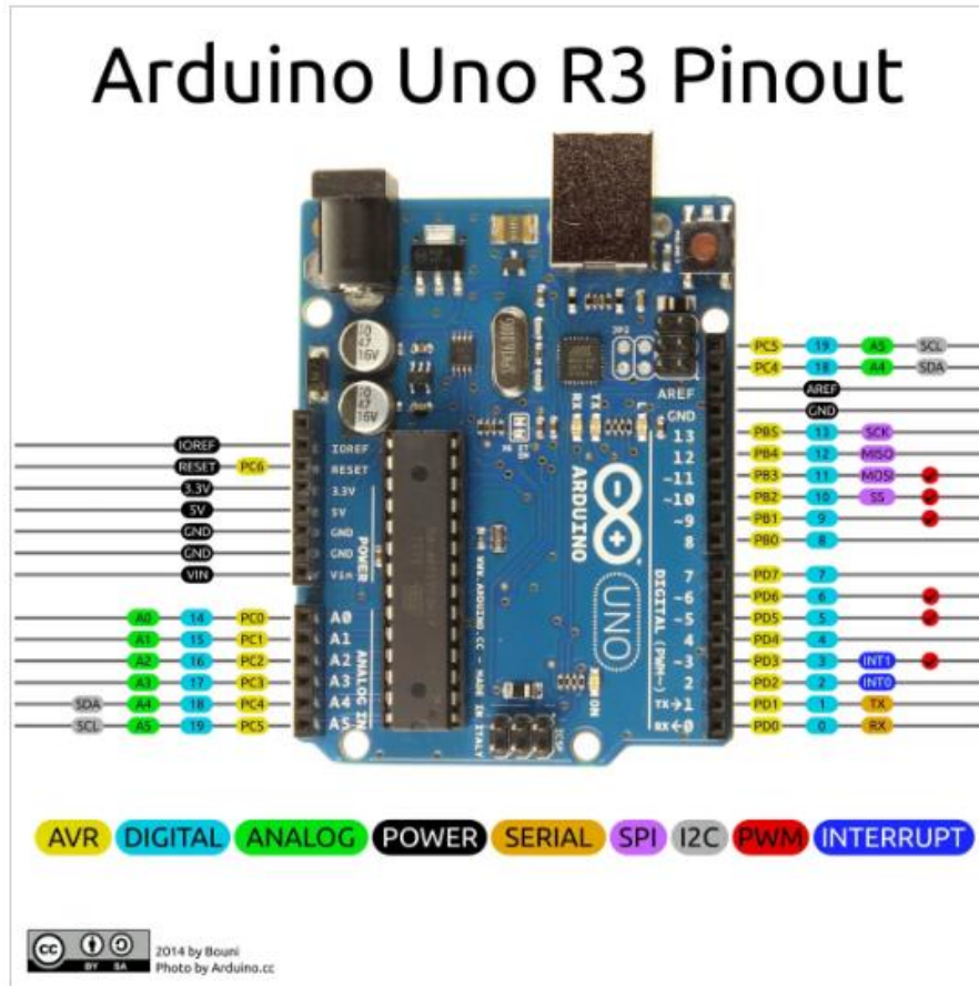
Figure B-3-1. Arduino Uno Pinout [11]
